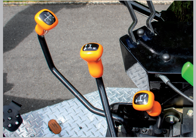
Latest transmission technology in a five-speed three range gearbox with underdrive.
