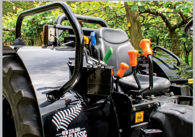
New hydraulic control arrangement and brush guard.
